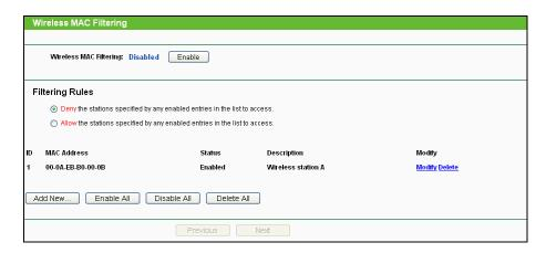
Figure 4-23 Wireless MAC Filtering
